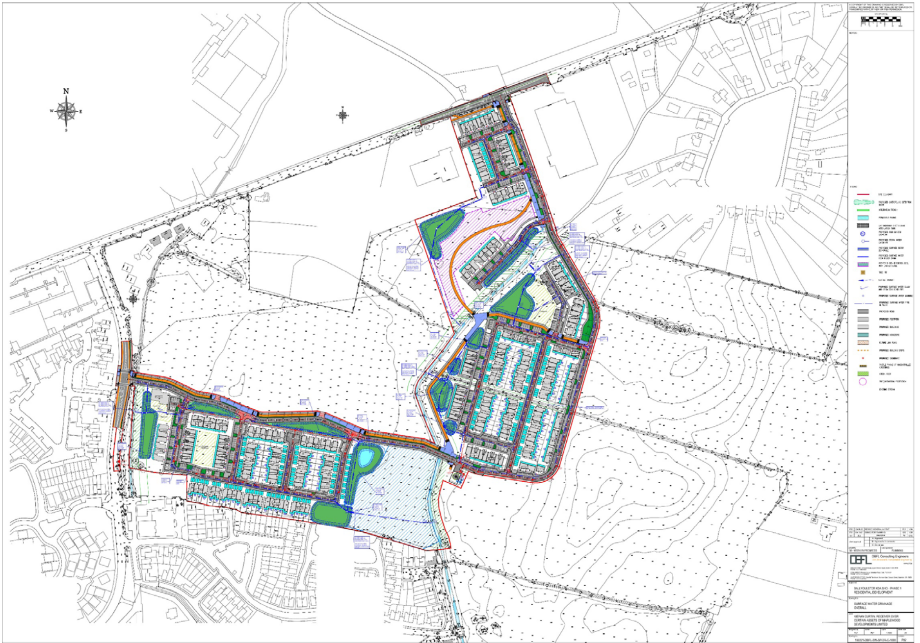
Figure 6. Surface water drainage layout - overall
